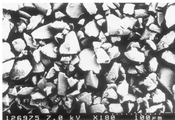
Fig. 2. SEM of molecular imprinted polymer particles prepared by traditional bulk polymerization and grinding-seiving-sedimentation procedures.
