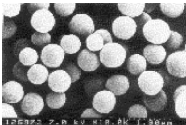
Fig. 3. SEM of blank microgel spheres. Molar ratio of MAA : EGDMA is 6.98 : 12, solvent (acetonitrile) fraction is 96% (v/v).
